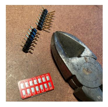
Line up the trimmed pins with the surface pads on the back side, making sure the vertical pins are aligned with circles. Solder both header pins in place, being careful not to melt too much solder onto the pads. Not a bad idea to check with a multimeter that no pins are shorted together.
