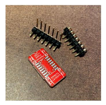
Using this style of <u>right-angle head pins</u>, trim the long legs down so they won't interfere with the opposite side.
