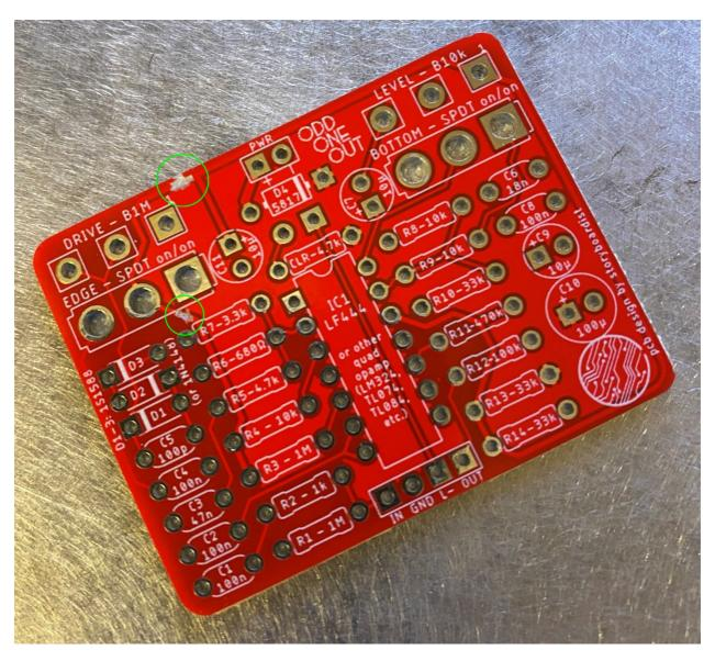
Use a multimeter and test that there's no connectivity between the middle pad/lug of the Edge switch and the top/square pad of C11 or the outer pad of R4. This disconnects the edge switch from the VR.
